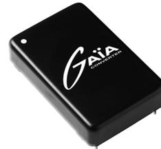
The input bus conditioner FLHG-60 designates a 60W input bus front-end that enables and eases construction of power architectures for military and avionic 24V and 28V applications. The FLHG-60 includes:
